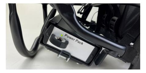
To remove the power pack, the tension lock on the bottom must first be opened. The power pack can then be pulled out by pulling it forward.
