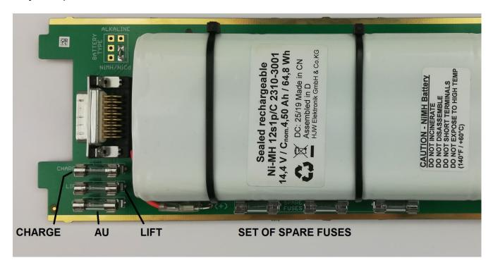
All input- and output connections are fused: Charge Input (CHARGE, 4 A slow-blow), Antenna Unit Output (AU, 1 A slow-blow) and Lift Output (LIFT, 0,5 A slow-blow). Additionally, spare fuses are provided.
