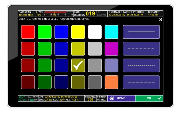
Mark a color field and a line style field and confirm with "OK".
