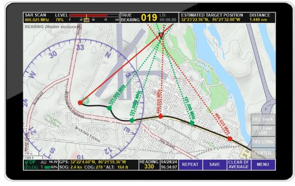
As with normal bearing mode, Lines of Bearing can be kept on the map by tapping "SAVE", with exception of those originating from 406 MHz (COSPAS-SARSAT) transmissions, which are saved automatically (Also refer to the chapter "Basic Elements and Functions of the Map Section").
