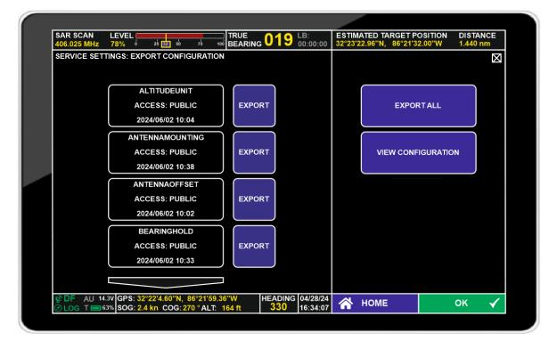
Files are stored in the mass storage device (e.g. SD-Card) under Android/data/com.rhotheta.rt400/files/Configurations. Each configuration item is stored in a separate file.
