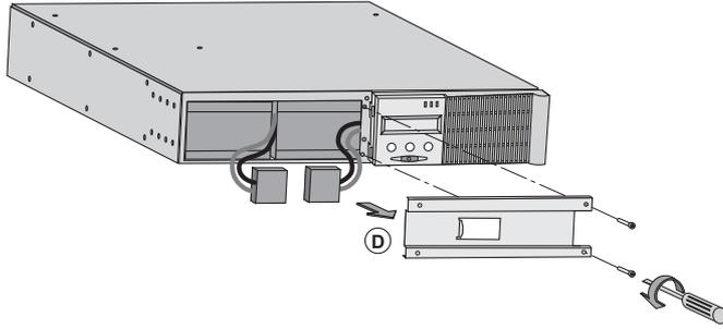
**D** - Remove the metal protection cover in front of the battery (two screws).
