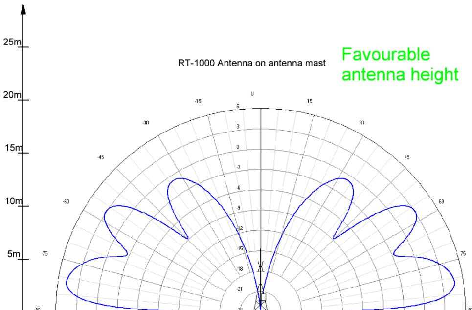
Ground reflections will cause the vertical antenna diagram having zeros, i.e. angles at which the sensitivity of the antenna is extremely low. Higher antenna positions cause more zeros in the vertical antenna pattern.
