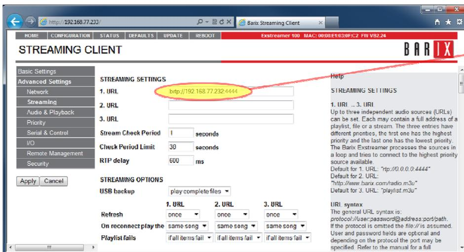
Please input here the accurate source IP address of the RT-1000 Multichannel audio module and the used Port.
