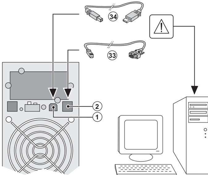
1 - Connect the RS232 (**33**) or USB (**34**) communication cable to the serial or USB port on the computer equipment.
