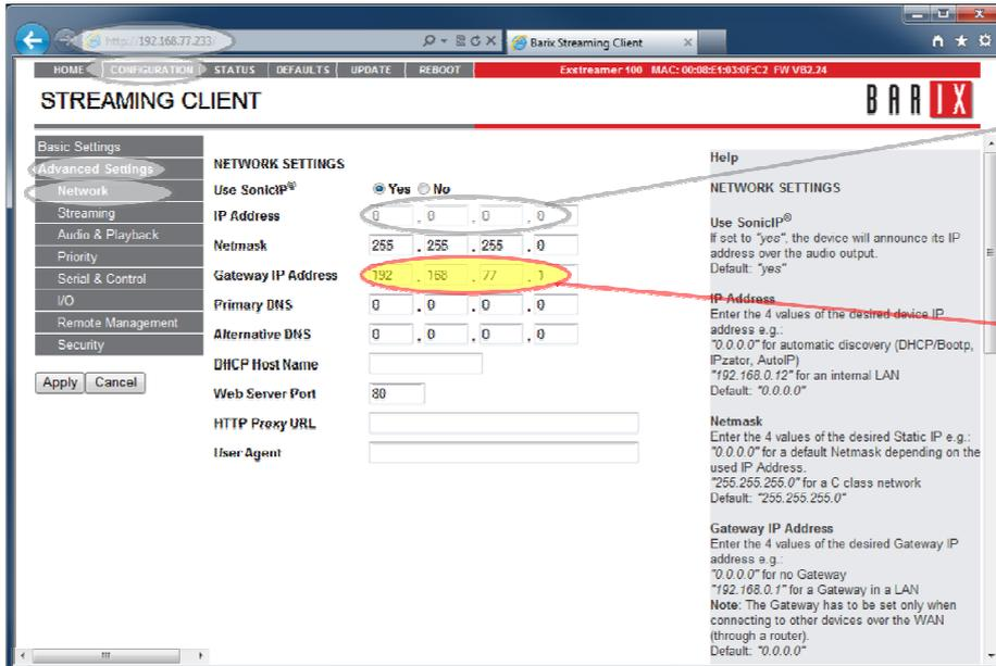
The IP address for this Ex-Streamer is preconfigured to DHCP.
